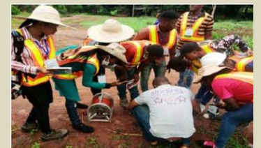
Fig 9: Cross-section of some participants carrying out electrical resistivity survey
