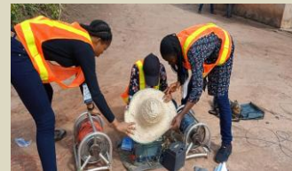
Fig 8: Some participants setting up the electrical resistivity meter in a station
