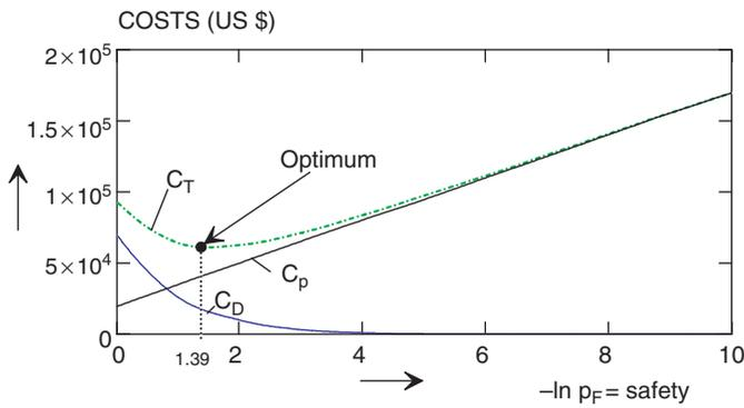
Figure 4 Total cost-reliability relationship for a flood levee.
