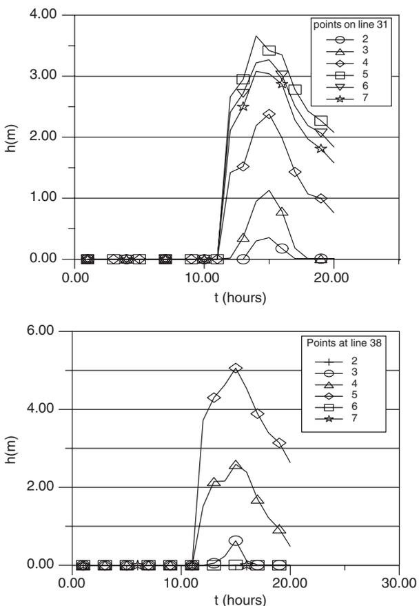
Figure 7 Water stage hydrographs  $h(t)$  at characteristic locations.
